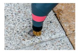
The Gum-e removes the gum with 230° F of heat in the steam, over 20% hotter than other steam machines.
